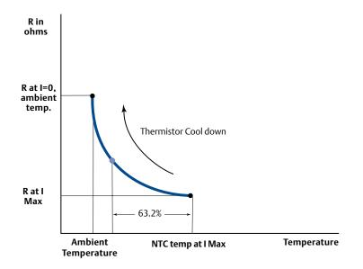
**Thermal Time Constant** – This is not how fast a thermistor will respond to a change in temperature. It is a method of comparing the relative speeds of thermistors with each other. By definition, the thermal time constant is the amount of time required for a thermistor to change 63.2% of the temperature difference between its initial and final sensing temperatures in a step-function change in temperature. This value is dependent on the sensing medium – still air, moving air, liquid, etc.
