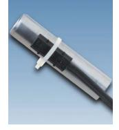
**Interfacing NTC Thermistors** – Thermistors require control circuitry to act on a power circuit. To replace a bimetal thermostat, a thermistor requires a few fixed resistors and a transistor/power semiconductor as a minimum. Since thermistors are solid state, they are much less prone to fatigue and can last hundreds of thousands of cycles with minimal change in characteristics, providing very high system reliability.
